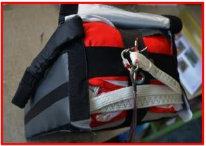
The rocket motor cable must be located under the forward flap. The length of the rocket motor rope must not be extended!
